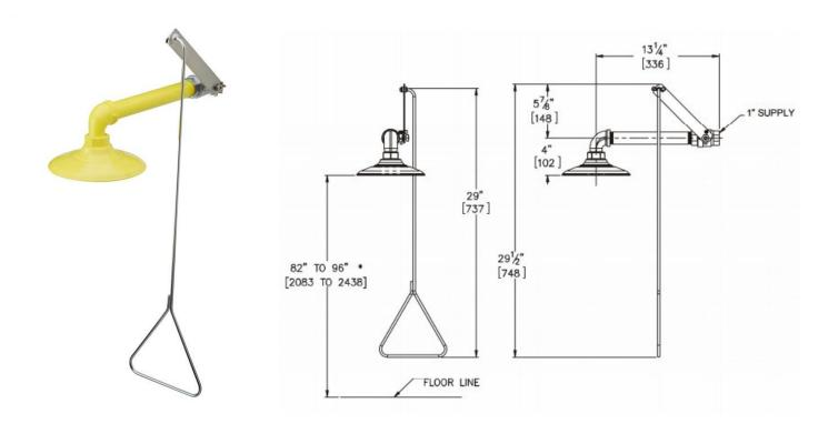
Model S1200 is our wall mounted safety shower with plastic head. Complete with plastic shower head, stainless steel pull handle and supplied with 1" chrome plated brass stay open ball valve.
